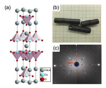
FIG. 1. (a) Crystal structure of the  $La_{2-x}Ca_{1+x}Cu_2O_6$ . (b) Asgrown  $La_{2-x}Ca_{1+x}Cu_2O_6$  single-crystal rods grown by the traveling-solvent floating-zone method. (c) Laue back-diffraction image of  $La_{2-x}Ca_{1+x}Cu_2O_6$  single crystal with (001) direction (c axis) pointing along the x-ray beam. Color points in (c) correspond to the calculated diffraction pattern, generated by software QLaue [22].
