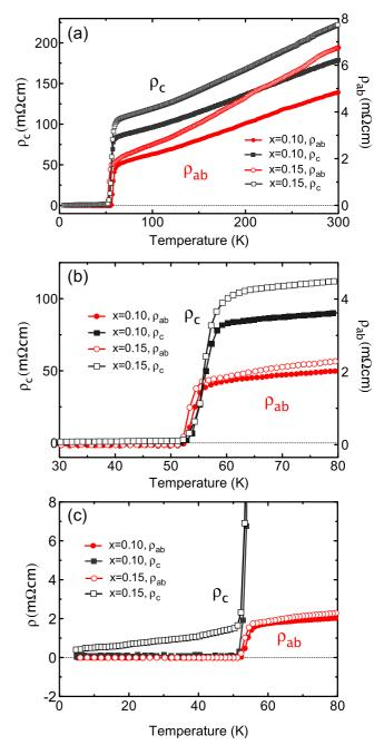
FIG. 4. (a) The in-plane resistivity  $\rho_{ab}(T)$  and interlayer resistivity  $\rho_c(T)$  of the superconducting  $\text{La}_{2-x}\text{Ca}_{1+x}\text{Cu}_2\text{O}_6$  single crystals. Different y-axis values are used to illustrate the normal-state resistivity in both directions. (b) A zoomed-in figure showing the superconducting transition near 54 K. (c) A zoomed-in figure showing the finite resistivity in  $\rho_c$  at low temperature.
